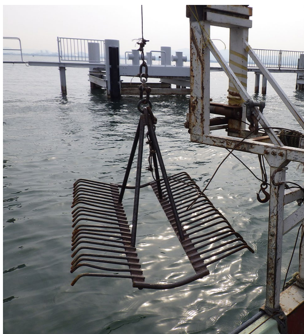
Fig. 2 Fork-shaped shellfish collecting gear, the ‘Man-gan,’ modified to harvest submerged macrophytes in Lake Biwa (courtesy of Dr. Eiso Inoue)
